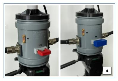
Remote tuning Compared to other antennas from BTV/LOOPER SYSTEMS production electric motor driving the air variable capacitor is not controlled by PWM using CB4M units. Simpler system is used, where fast and slow
